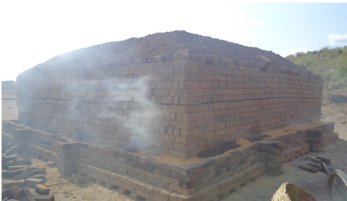
Figure 6: Burning the bricks with husk and coal which is polluting the environment
